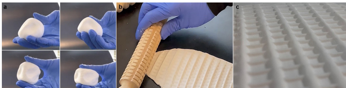
Figure 1. a) Hand-rolled yttria-stabilized zirconia (YSZ) dough, b) a showcase on the possibility of roll-to-roll processing, and c) imprinted features.
