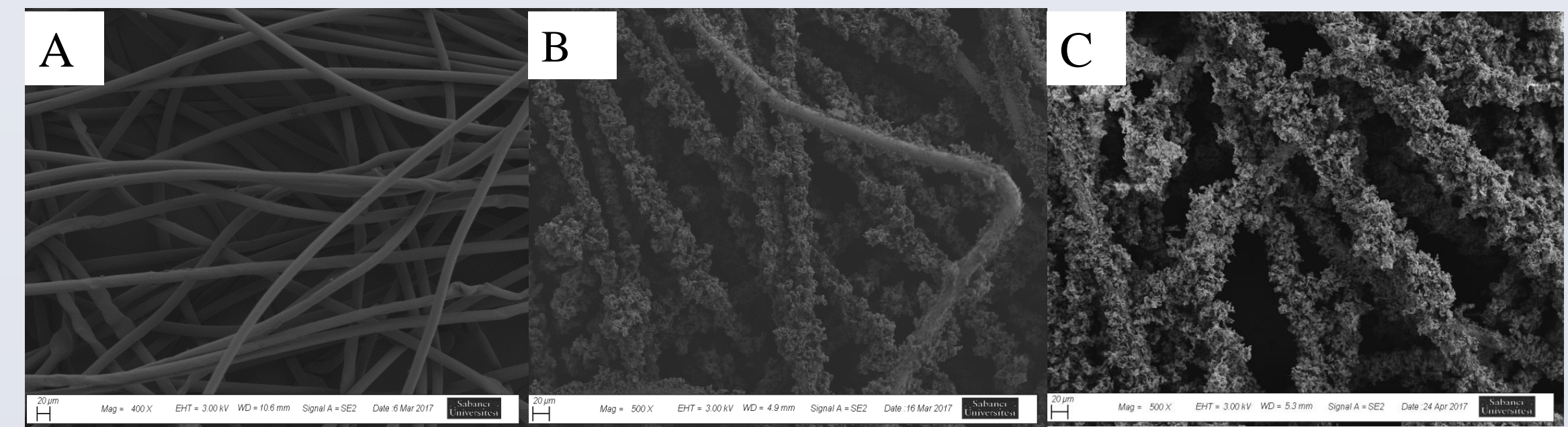
A) SSS nonwoven Electrospayed with B) 25µl/min 4 hour (N6) C) 25µl/min 8hour (N8)
