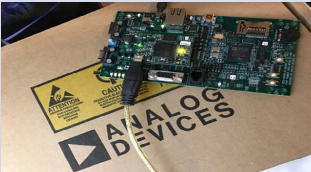
Fig. 2. Blackfin BF609 DSP module for producing real time radar signals
