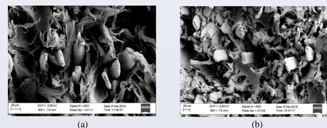
During the SEM studies of wood fiber added PP with and without compatibilizer addition, the effect of compatibilizer on the homogeneity of the compound is analyzed. When the breaking surface of the mechanical test bars are studied under SEM, it is observed that PP with compatibilizer addition shows a more homogeneous structure.
