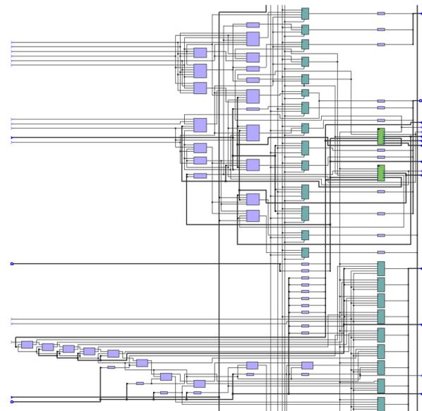
Figure – 4: Snapshot of synthesized Binarization module with Quartus Prime
