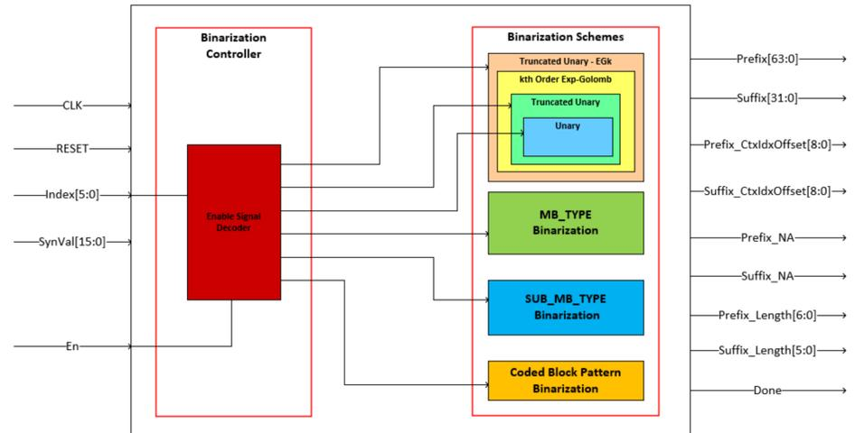
Figure – 3: Hardware Model of Binarization Module
