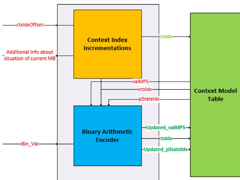
Figure – 2: Software Model of Context Modeler and Binary Arithmetic Encoder
