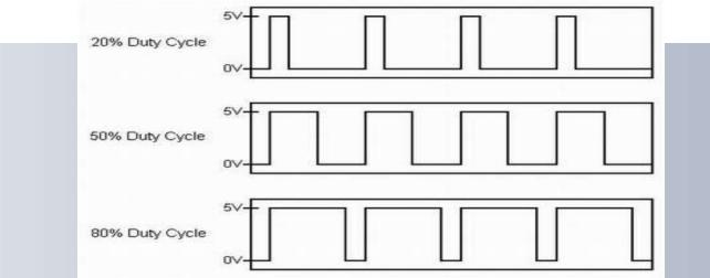
Figure above is a generic PWM signal at different duty cycles, a duty cycle is the percentage of time the signal is on compared to off. As duty cycle increases, the signal is on for longer, thus increasing total power.
