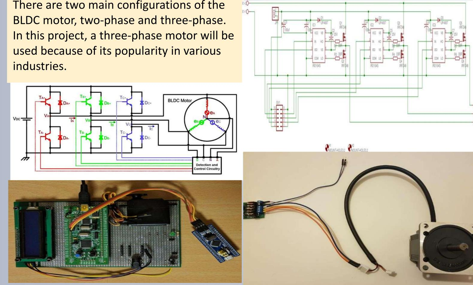
You can see our motor driver. It includes 6 pieces of Mosfet, 3 pieces of half- bridge driver and other necessary electronics (resistors, diodes, capacitors) materials. We have achieved the necessary power by making these connections one by one. Our card that has been used in our preliminary design was designed and built by Dr. Onat. It has 5 cable connections, two of them are connected to power and the other three are connected to the BLDC motor.
