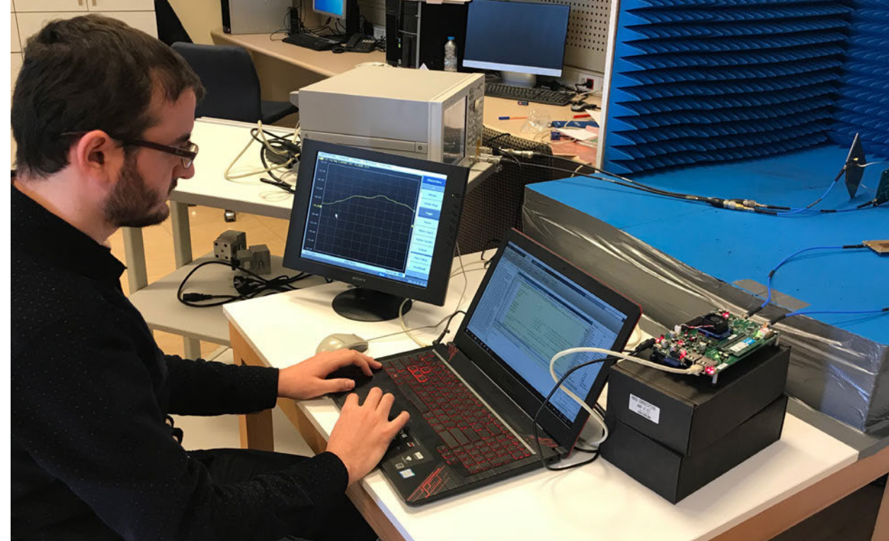
FD radio development and test set-up
