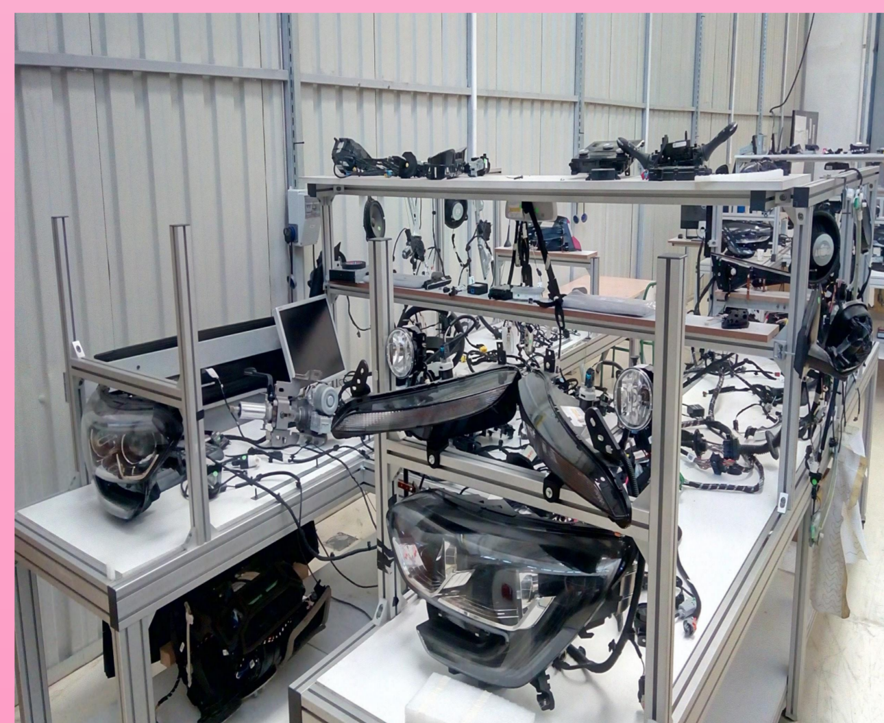
Fig.2 An example of wire harness test bench
