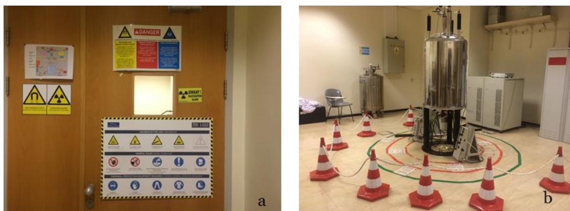
Figure 15.2 NMR room warning signs (a), NMR spectrometer warning signs and bands (b)
