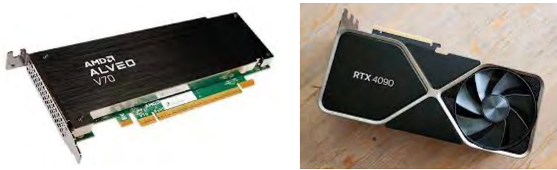
Figure 2. Two commonly used hardware accelerators for diverse applications: FPGA (left) and GPU (right).
