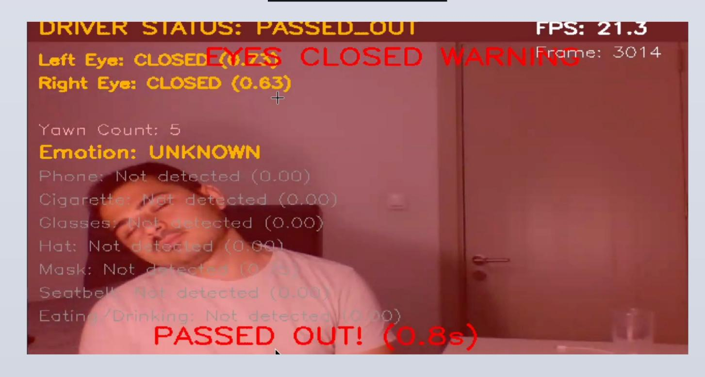
The system monitors various visual indicators such as eye openness, head position, and the presence of objects like phones, cigarettes, glasses, hats, and seatbelts. It outputs the driver's status (e.g., "DISTRACTED", "NORMAL", or "PASSED-OUT") based on real-time object detection and fatigue classification.
