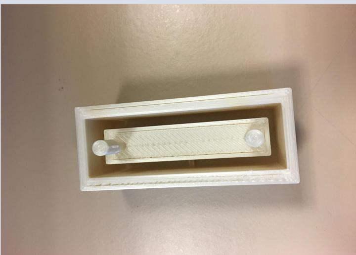
This device will allow us to analyze the migration rates of cells in 3D format. It is known that cells act differently when they are in 3D format. The mold in the figure above will be used for the experiments.
