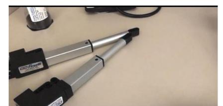
Firgelli L12 LEGO NXT 50mm linear actuators
